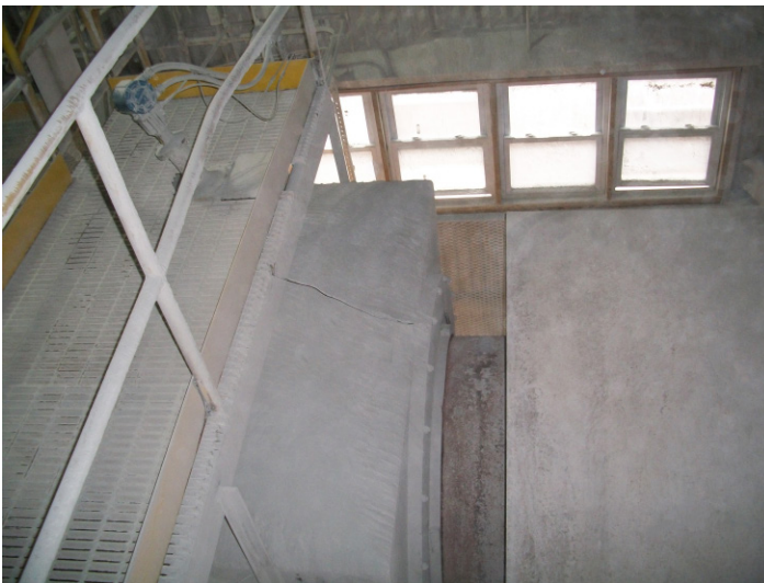
Figure 3 - Long probe inserted down through feed box
