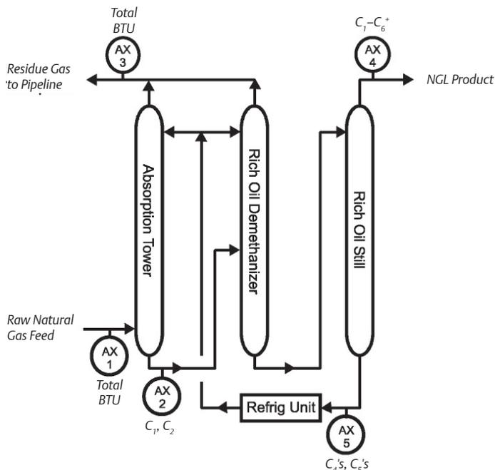
The stripping oil plus any of the heavy components from the natural gas enter the rich oil still where the natural gas liquids are boiled out of the stripping oil. This natural gas liquids product stream is then sent to a natural gas liquids plant for further separation or is sold to a chemical plant as feedstock.
