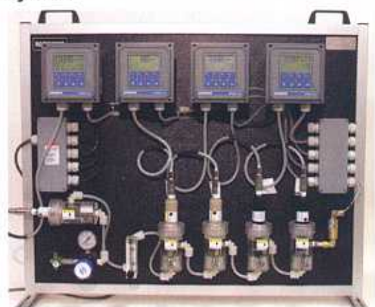
Photo 1. Electrochemical water quality monitoring system ensures water safety and quality throughout the distribution system
