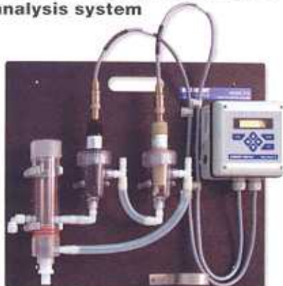
Photo 3. Analytical systems directly measure monochloramine without chemical reagents to condition the sample
