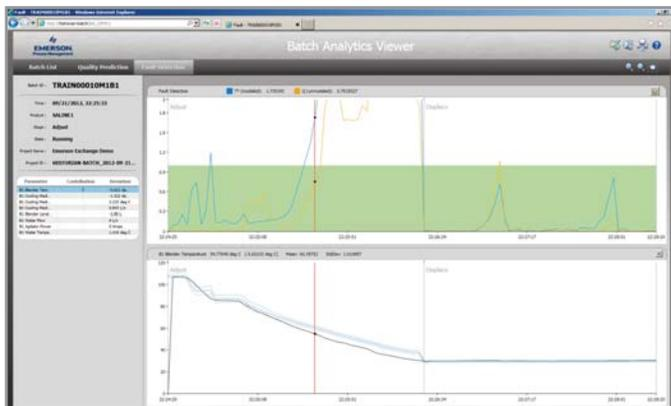
*Batch Analytics' web-based interface makes it easy for the operator to see immediately where a problem is occurring. In the example shown, a variable is trending below the level indicated by the model.*
