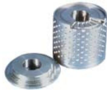
The Fisher Severe Service group replaced the eroded valve with a new valve incorporating a characterized Cavitrol® III trim. The three-stage trim was designed to meet both the initial startup demands (when there is potential for cavitation) as well as capacity requirements. The new valve body was made of WC9 chrome-moly material to enhance its corrosion resistance.
