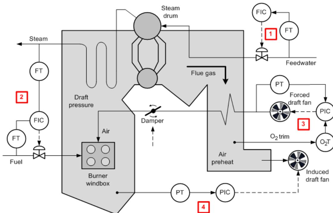
Figure 11: Generic basic boiler controls on balanced draft type configuration<sup>3</sup>
