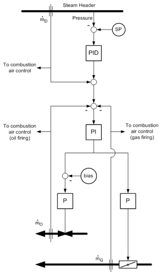
Figure 9: Typical control scheme for firing natural gas and oil<sup>17</sup>
