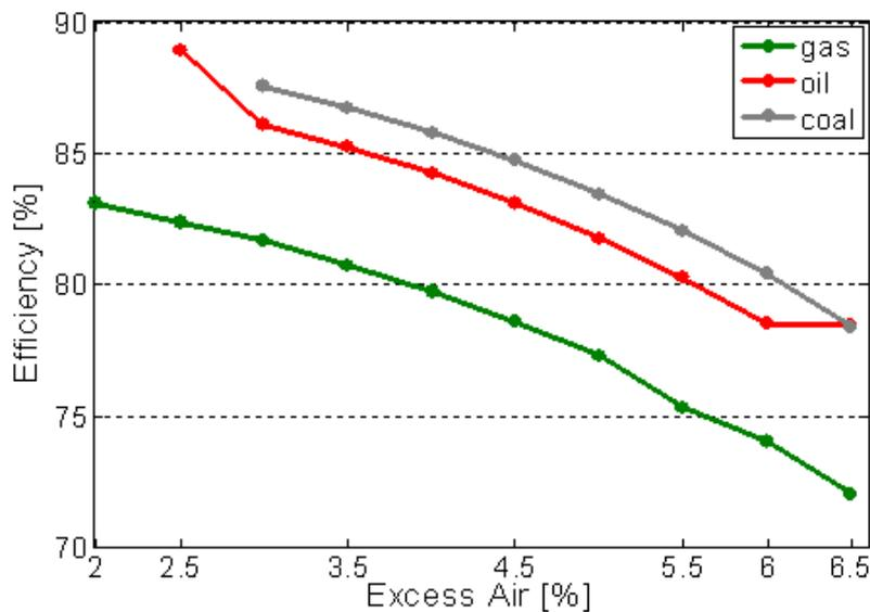
**Figure 4: Boiler efficiency vs. excess air in large boilers<sup>5</sup>**
