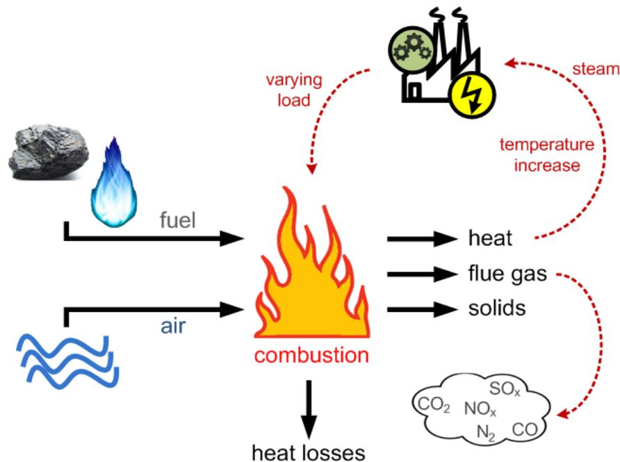
**Figure 1: Heat generation through combustion**
