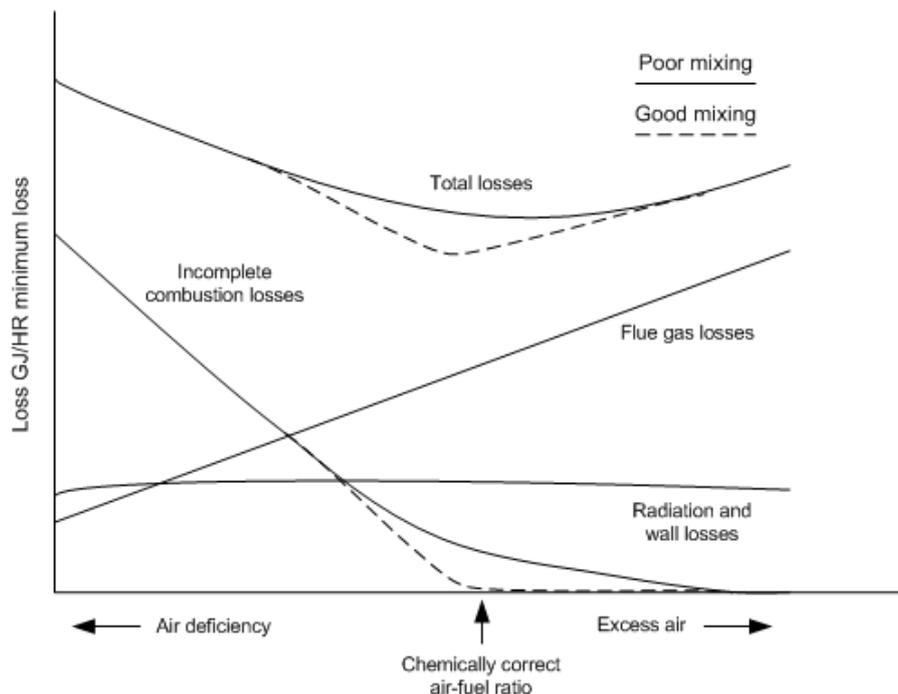
**Figure 5: Operational trade-offs vs. excess air levels<sup>5</sup>**
