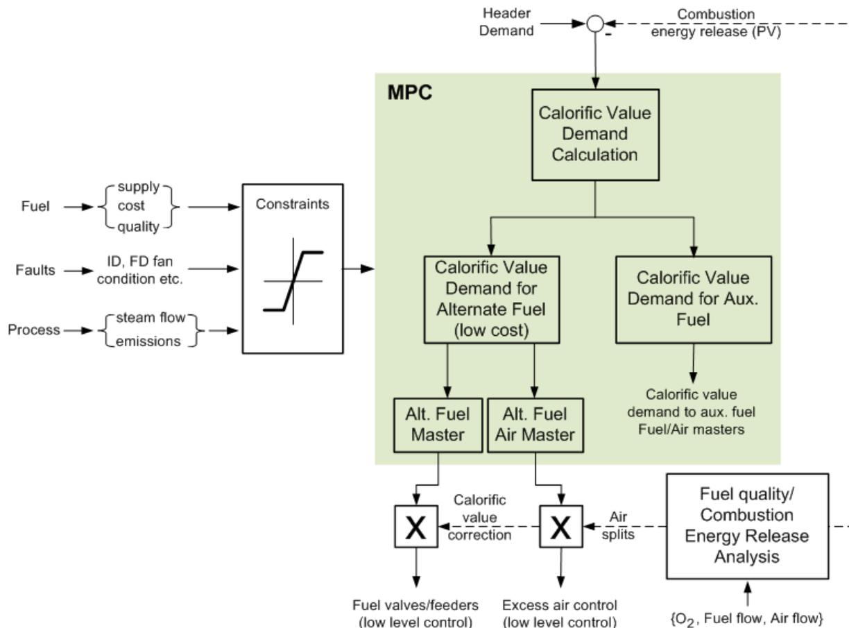
**Figure 15: SmartProcess Boiler strategy rearranged in a feedback control formulation**
