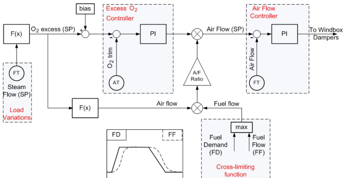
**Figure 16: SmartProcess Boiler Air flow control and cross-limiting**
