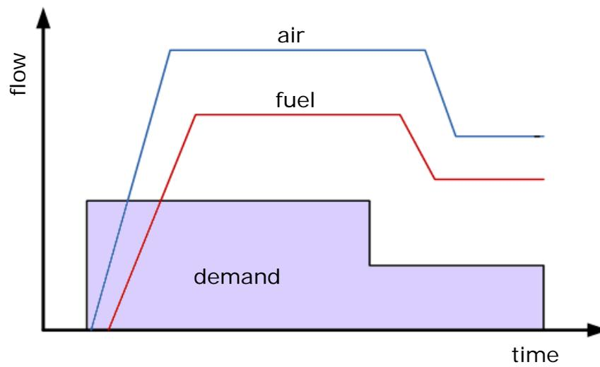
Figure 13: Cross-limiting effect during load changes
