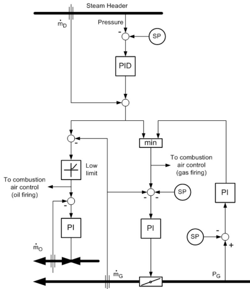
Figure 10: Method for fuel burning prioritization<sup>17</sup>
