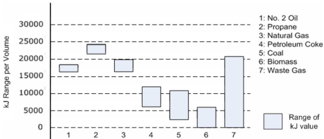
**Figure 8: Fuel calorific content variations<sup>15</sup>**
