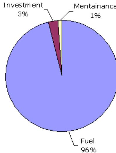
Figure 6: Full load steam system costs breakdown<sup>9</sup>
