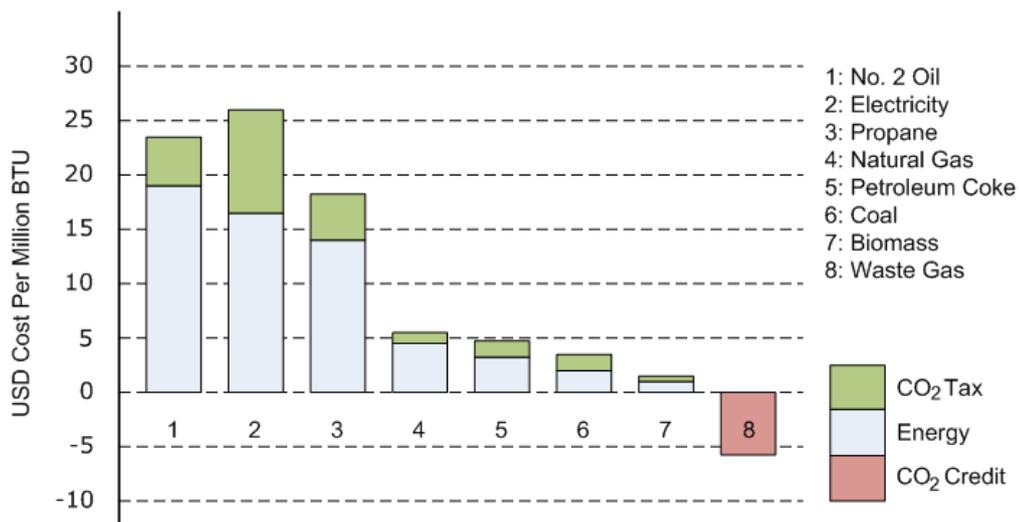
Figure 7: Fuel Cost Including CO<sub>2</sub>
