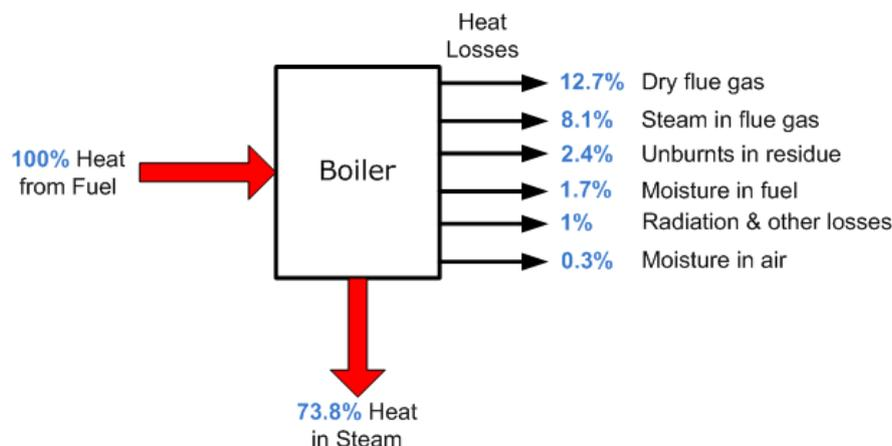
Figure 3: Typical Industrial Boiler losses<sup>6</sup>
