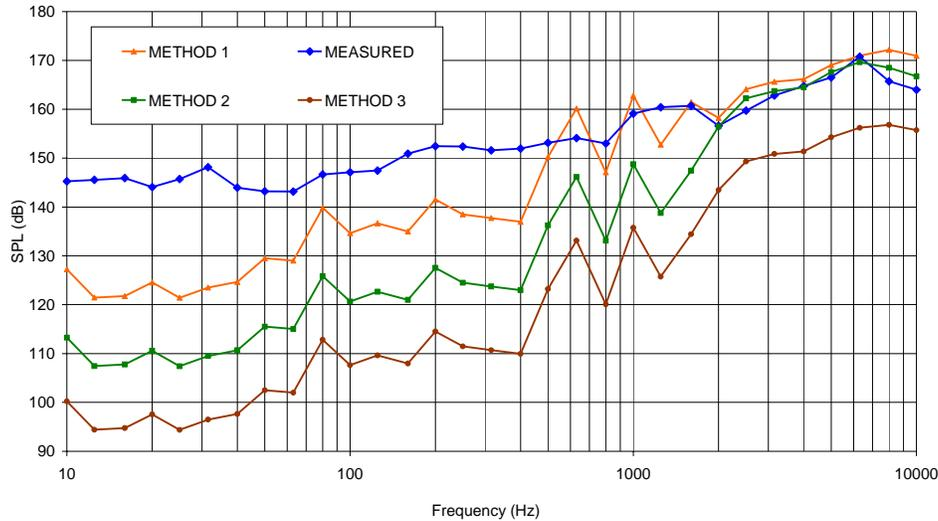
**Figure 6:** Comparison of the measured and predicted internal sound level.
