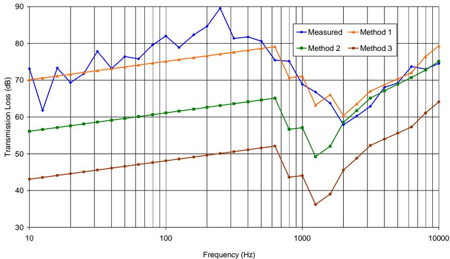
**Figure 5:** Comparison of the predicted transmission loss of the three methods.
