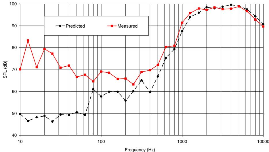
**Figure 3:** Comparison of the measured and predicted external sound level.
