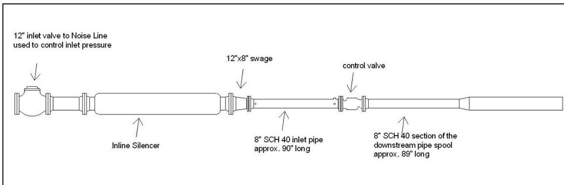
**Figure 2** Schematic of the flow line used for testing. 8" SCH 40 section on the far right was the test section and the control valve was the internal noise source.
