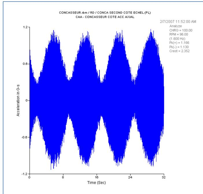
*The combination of a resonance problem with an outer race problem and an installation problem created this extraordinary waveform.*
