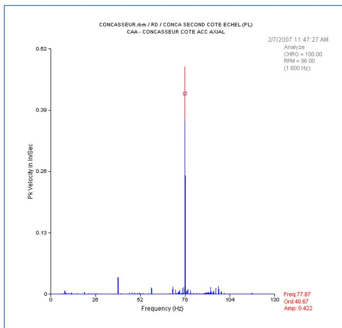
*On 7 February 2007, a very high frequency was measured at 78 Hz on a rotor in axial direction.*
