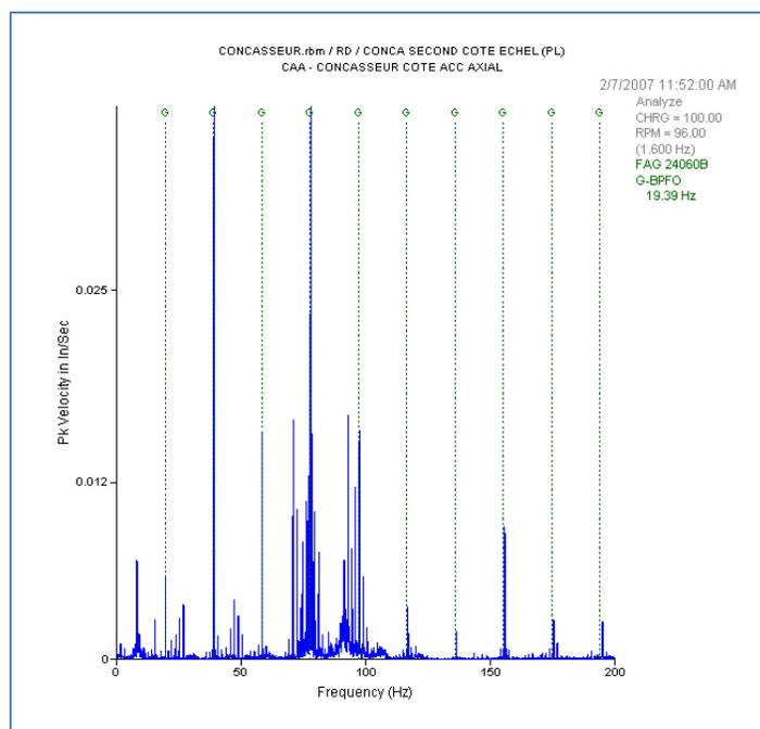
When we take a closer look at the spectrum in the neighborhood of 78 Hz, we see an increased floor level, which can be an indication of a structural resonance frequency. In other words, the 4th harmonic of the outer race problem has such high amplitude because it is amplified with a structural resonance.
