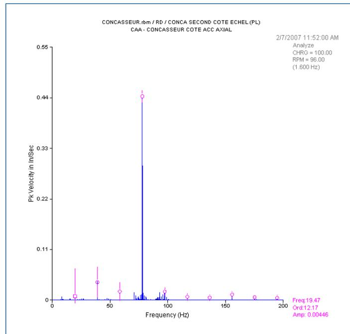
A closer look at the spectra shows us that there are 2 harmonic families in the spectrum, one at 19.47 Hz and one at 19.50 Hz. If we want to explain the beat frequency at 77.87 Hz and 78.0 Hz, we have to find an explanation of 19.47 Hz and 19.50 Hz.
