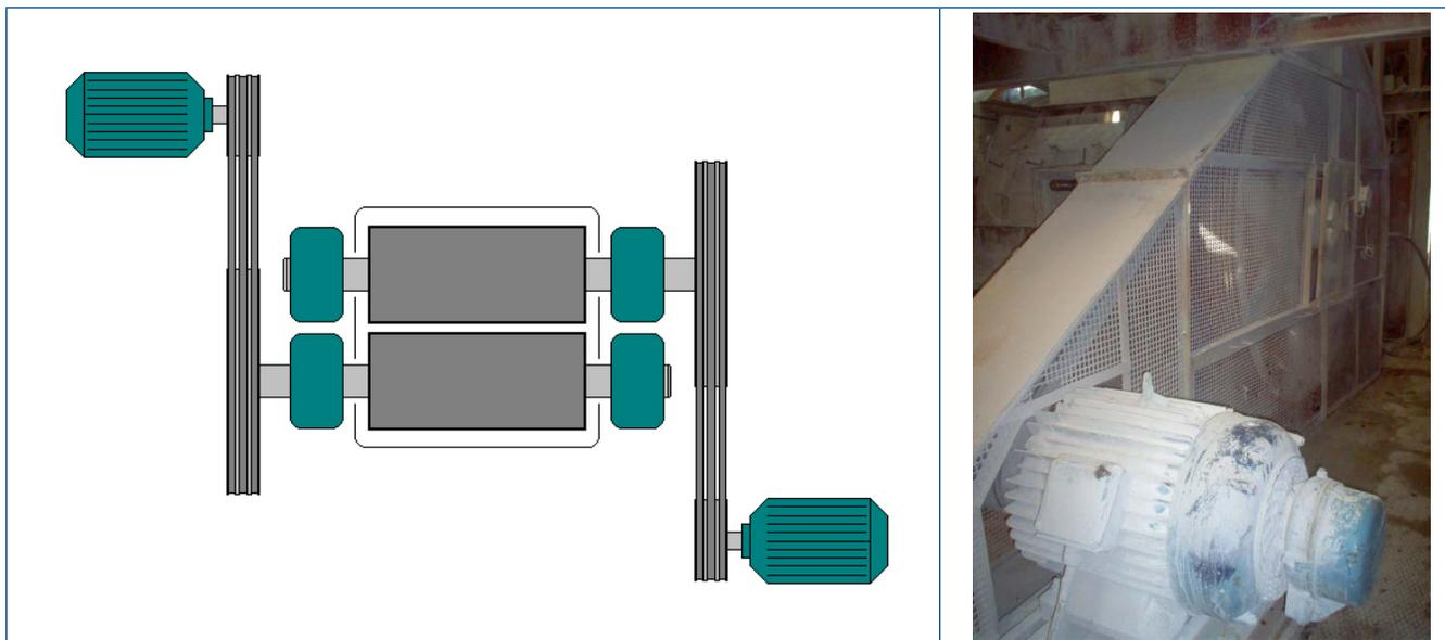
The installation is a concrete breaker. 2 motors with a speed of 740 RPM are connected with a belt to roll with a speed of 100 RPM.
