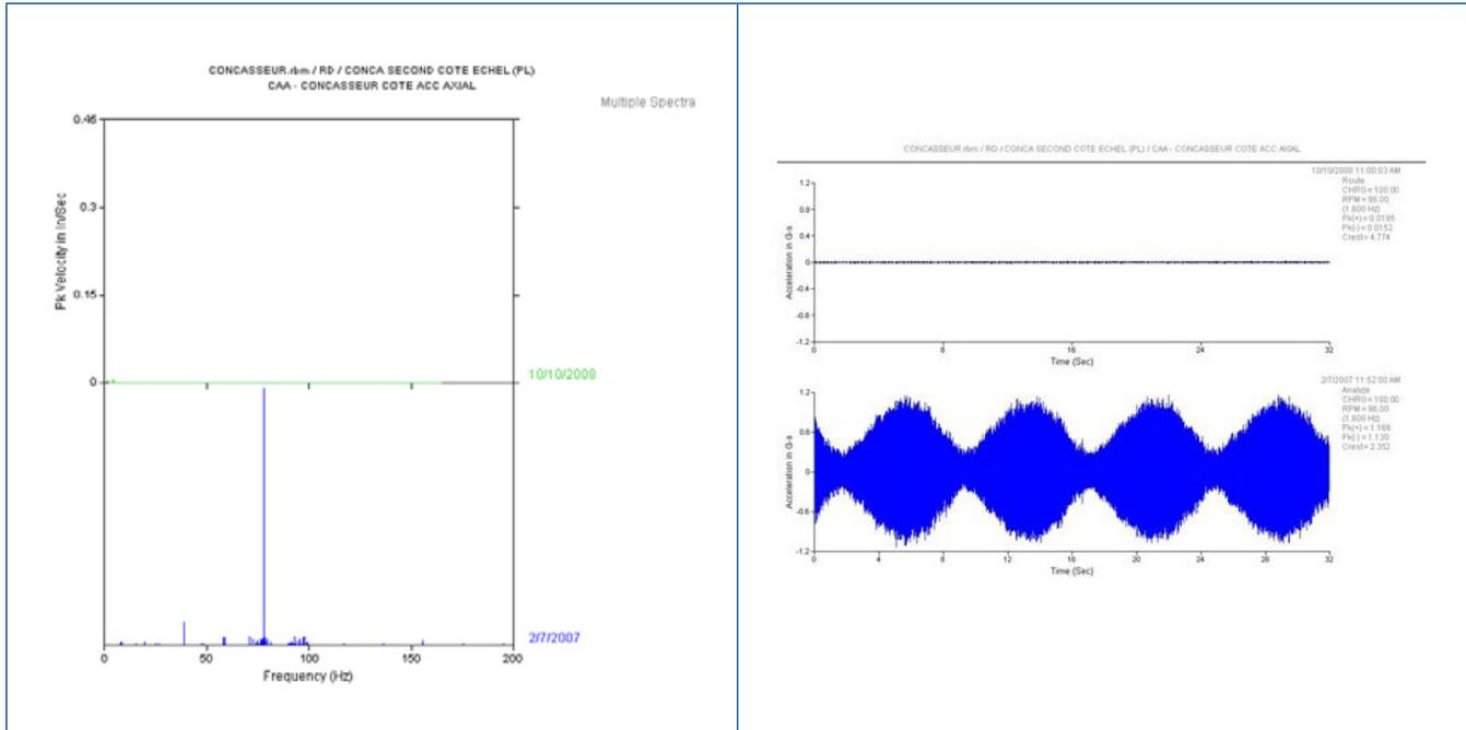
The last pictures show a comparison of the spectra and waveforms before and after the bearing replacement.
