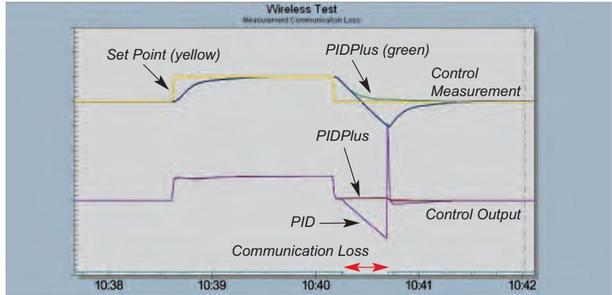
**Figure 4.** PIDPlus and traditional PID respond to a set-point change followed by interrupted wireless measurement updates. Note that in a real-life situation, process-value data would not be available during communication interruptions.
