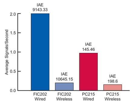
**Figure 1.** The average number of signals transmitted per second by measuring devices in two closed-loop scenarios, alongside integrated absolute error (IAE) values. Wireless devices measuring a flow-control variable using the report-by-exception communications scheme transmit about one-tenth as many signals as wired devices using the standard scheme. While measuring a pressure-control variable, report-by-exception transmits about one-sixth as many signals. IAE is comparable in both scenarios.
