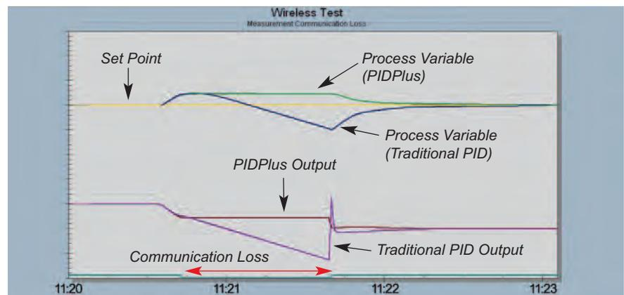
Figure 3: Simulation of a process disturbance, with controller input interrupted by a loss of communications. Note that in a real-life situation, process variable data would not be available for the entire period.
