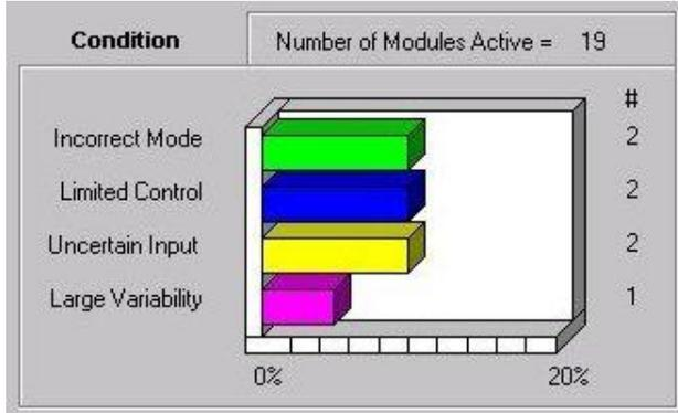
The modules included in this summary are also individually listed. By selecting one of these modules, you get a detailed view of the input/output, or control blocks in the modules that are malfunctioning. You can also view the calculated variability and percentage of time an abnormal condition existed.
