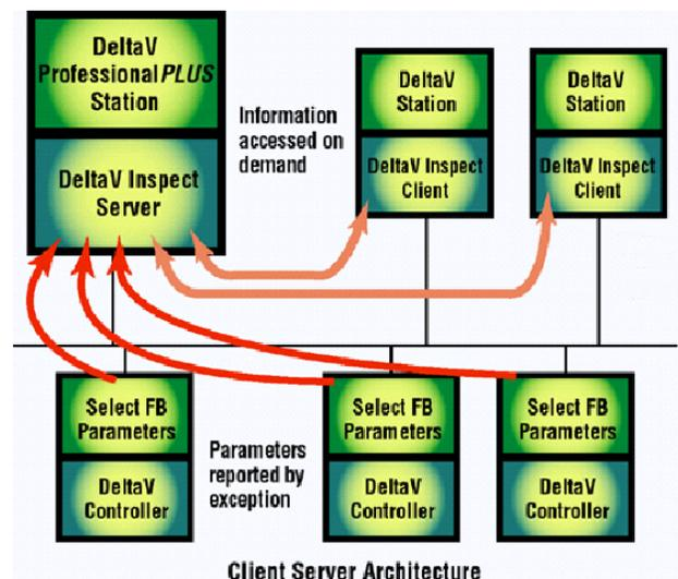
Based on block mode and parameter status, DeltaV Inspect automatically identifies abnormal conditions and graphically displays them on a DeltaV workstation. The conditions detected are:
