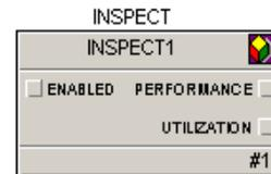
The Inspect block also allows you to historically trend and even alarm on the performance or utilization parameters for a given process area or the entire system.
