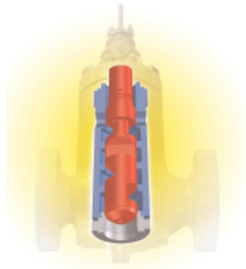
DST and NotchFlo® DST solutions, ranging from 1- to 4-inches, were utilized in the Cold High Pressure Separator system. Each of these designs combat damaging cavitation and flashing while allowing particulate up to 1/2-inch in diameter to pass without plugging the trim.
