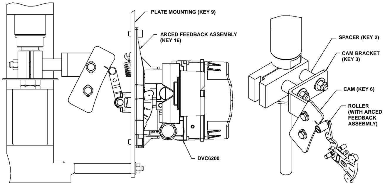
Figure 2. Installing CAM and Roller Feedback Assembly
