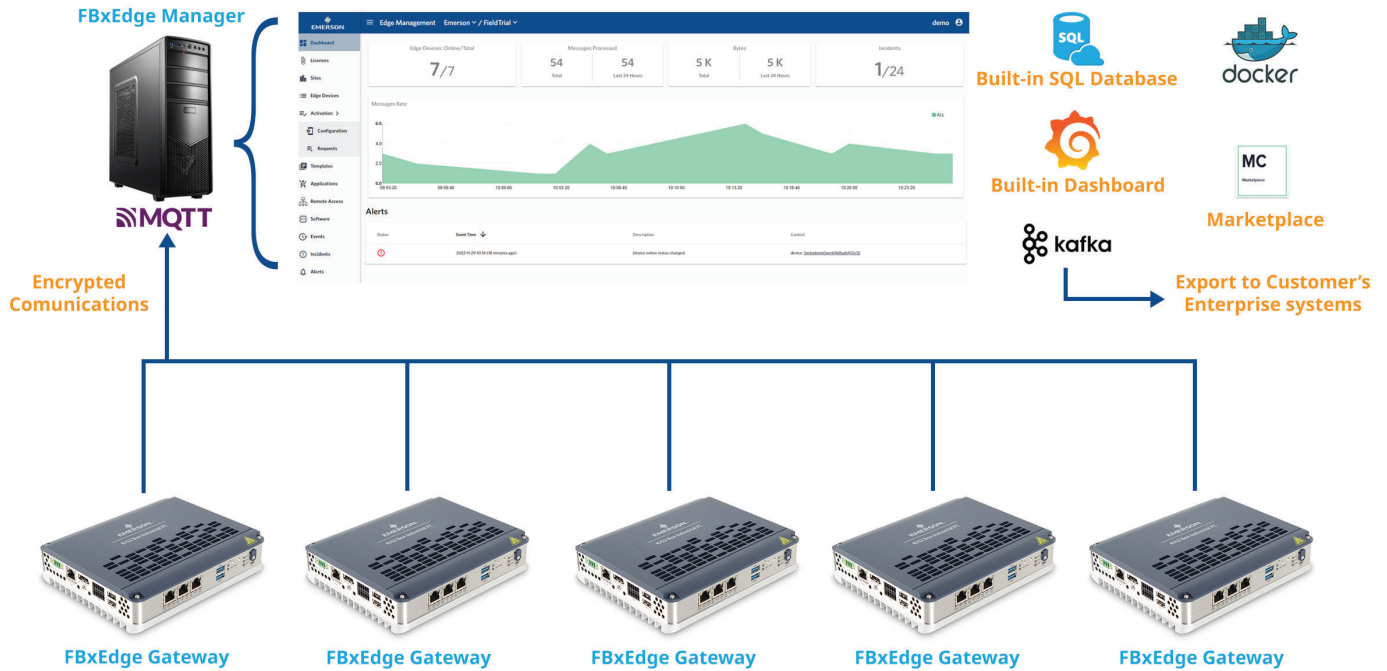
Figure 8: FBxEdge Manager enables FBxEdge users to leverage powerful central management capabilities, including bulk deployment of tags, applications, and remote upgrades.
