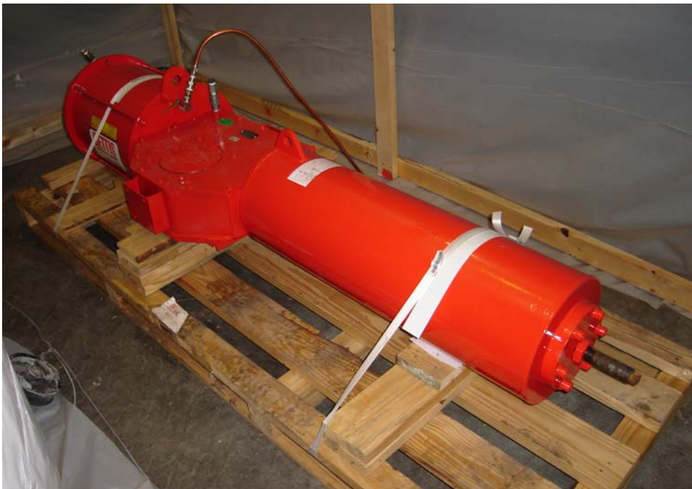
Photograph No. 2 View of the Actuator inside Dust Test Chamber
