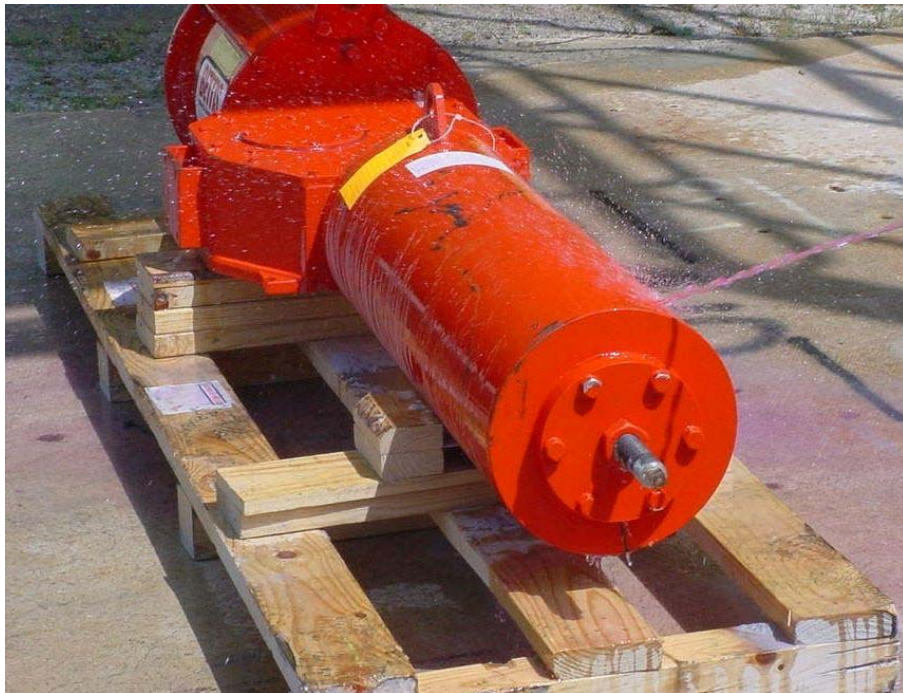
Photograph No. 6 Water Penetration – Powerful Jetting
