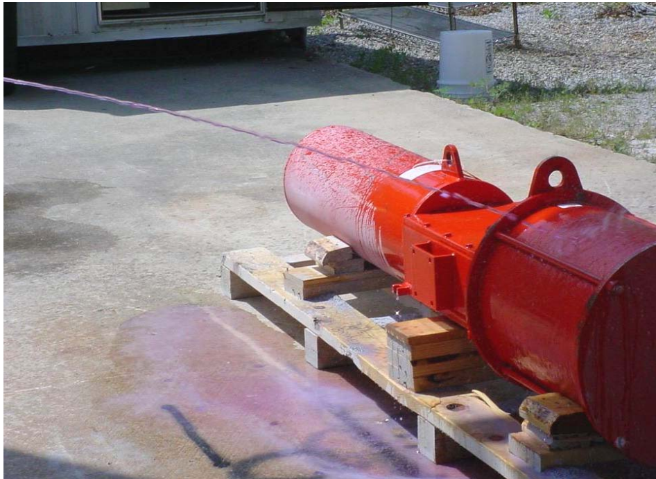
Photograph No. 7 Water Penetration – Powerful Jetting
