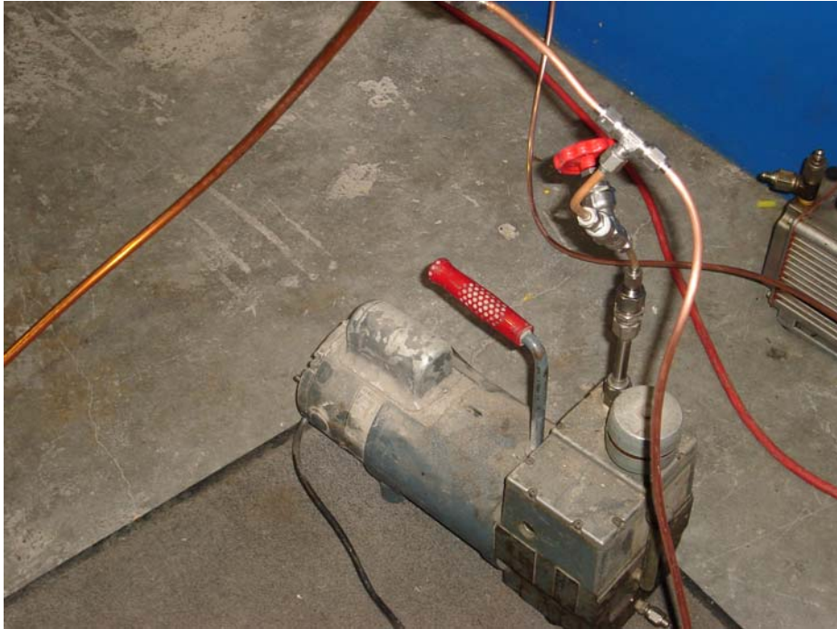
Photograph No. 3 View of Vacuum Pump for Dust Testing
