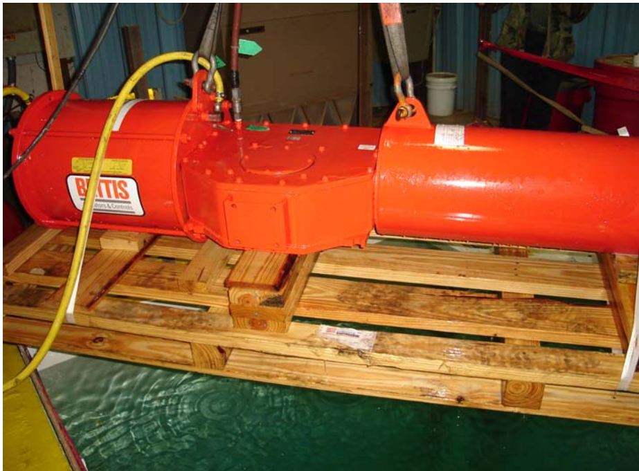
Photograph No. 10 Water Penetration – Immersion Test
