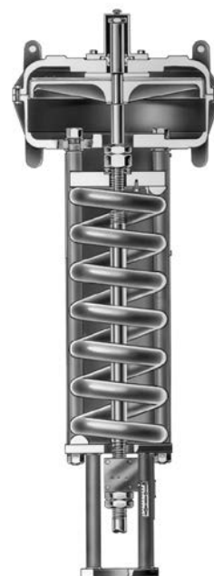
Figure 1. Sectional view of Fisher 657 Size 100 Actuator
