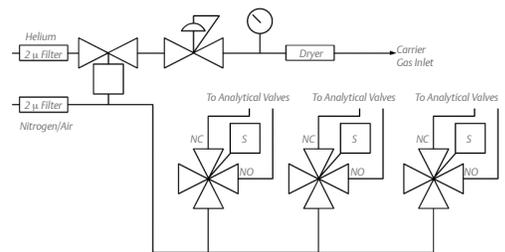
Figure 2 shows the flow path with the alternative actuation gas kit installed. The pneumatic shut-off valve will shut-off the flow of carrier gas in the event of the loss of actuation gas pressure. Without this shutoff, if the actuation gas pressure falls none of the pistons in the analyzer valves will seal. This will create multiple paths for the helium to escape to vent and dramatically increase the use of helium use, possibly emptying the helium supply.
