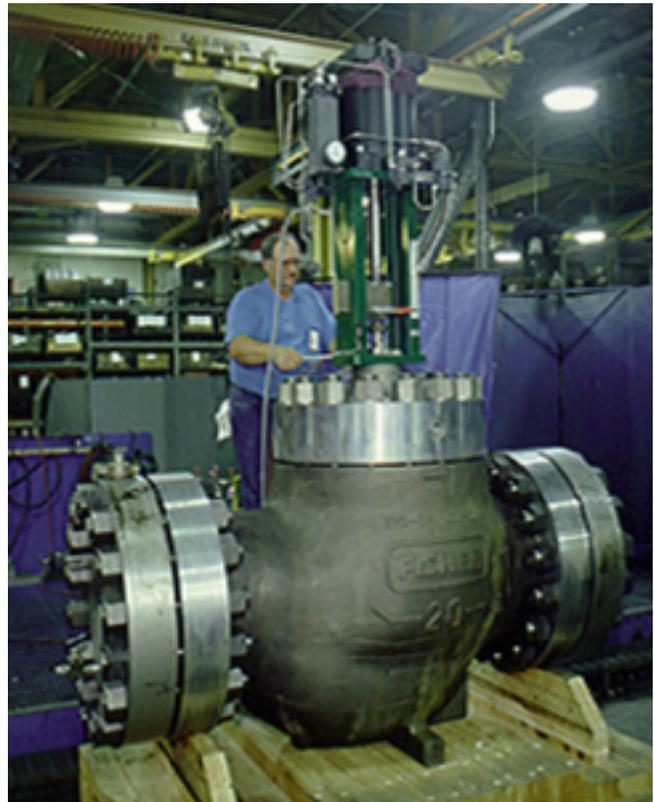
Because of its large size, the valve was a challenge to manufacture. The Fisher Severe Service Group in Marshalltown, Iowa, USA provided valve body and trim designs and worked with Fisher manufacturing personnel to conduct radiography and magnetic-particle testing. While the average production lead-time for a valve with similar requirements is about 24 weeks, the Marshalltown manufacturing team shipped the valve within 11 weeks to meet a critical delivery deadline for the platform’s revamp.
