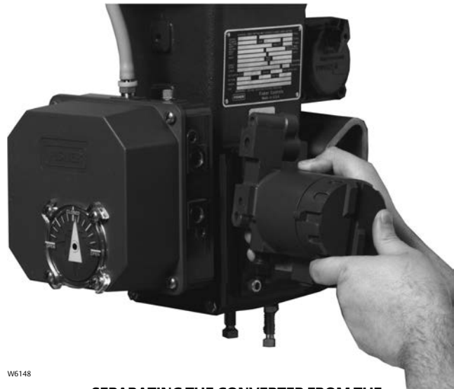
SEPARATING THE CONVERTER FROM THE POSITIONER BASE PLATE
