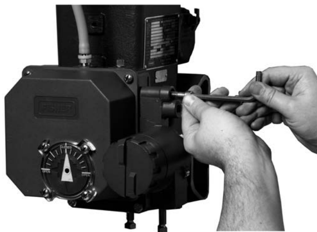
Figure 24. Removing the Converter Mounting Screws
