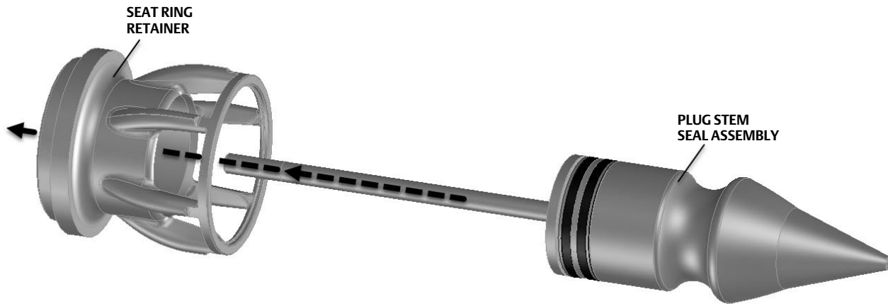
Figure 9. CCV NPS 4 Assembly - Insert of Plug Stem Seal Assembly through the Bottom of the Seat Ring Retainer
