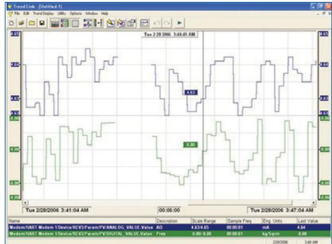
Leverage third-party trending applications through the OPC Server to view live instrument and valve data and access predictive diagnostics through AMS Device Manager.
