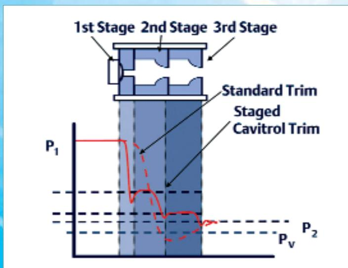
Figure 2. Staged pressure drop.
