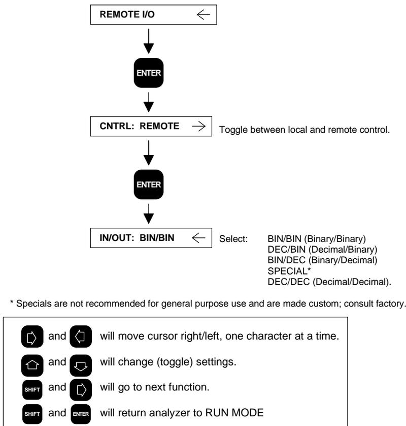
**FIGURE 3-16. REMOTE INPUT/OUTPUT**
