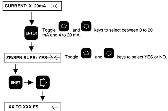
Note: Current Output is factory set at 4 to 20 mA. If an adjustment is needed, Zero and Span pots are located on the Power Supply Board.
