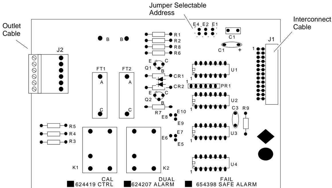
Note: The Dual Alarm, Fail Safe Alarm and Calibration Gas Control use the same board. However, the jumpers locations are different.
