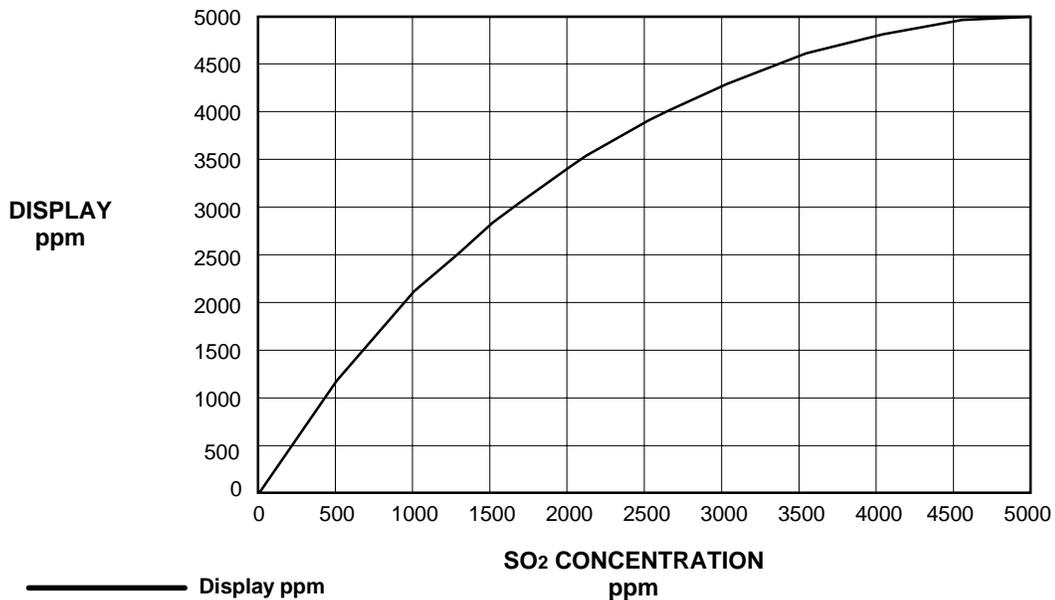
**FIGURE 3-9. TYPICAL APPLICATION LINEARIZATION CURVE**
