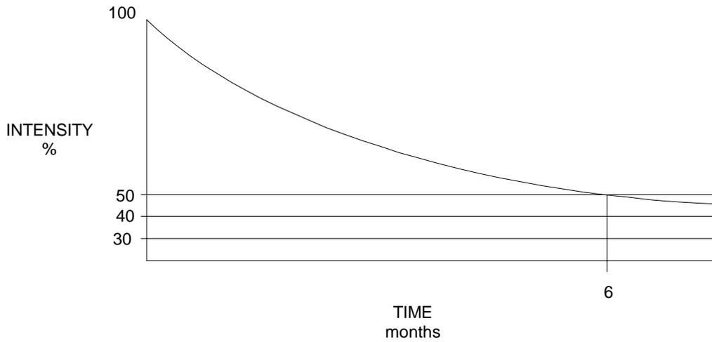
**FIGURE 7-3. UV LAMP LIFE VS. INTENSITY**
