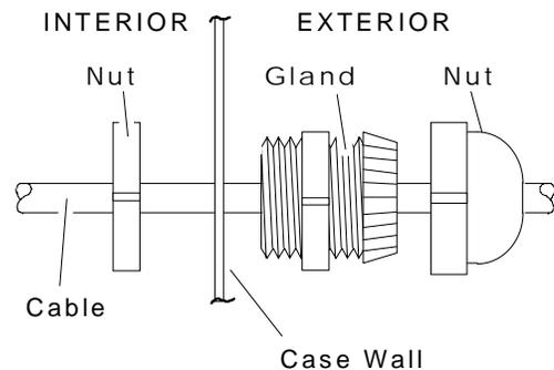
**FIGURE 2-2. CABLE GLAND CONNECTION**
