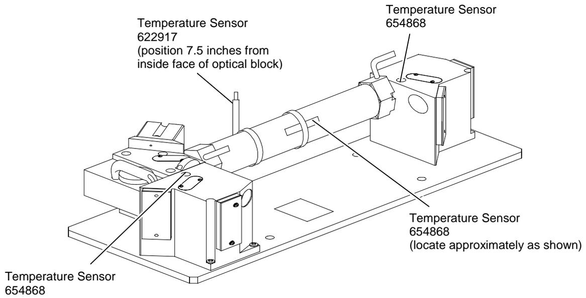
**FIGURE 7-2. OPTICAL BENCH - SENSOR LOCATIONS**
