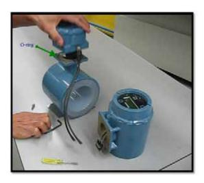
**NOTE**Make sure the terminal block openings are all the way open.
