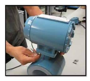
After all four bolts are installed and tightened, the installation is complete.
