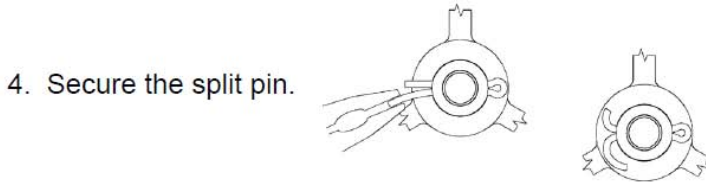
Figure 3 Mounting procedure for centering disc on rigid single lead probe (13 mm; 4B)
