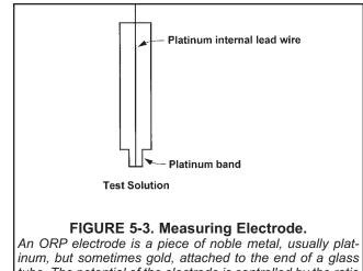
inum, but sometimes gold, attached to the end of a glass tube. The potential of the electrode is controlled by the ratio of oxidized to reduced substances in the sample. pH and other constituents in the sample may also affect ORP.
