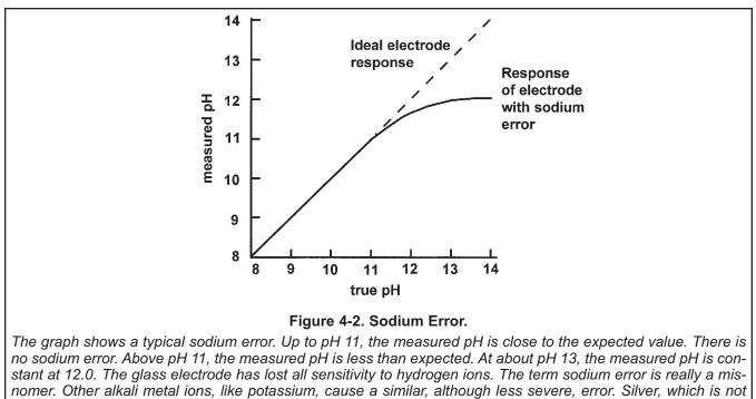
an alkali metal, also causes "sodium" errors.
