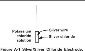
The electrode is a piece of silver wire plated with silver chloride in contact with a aqueous solution of potassium chloride.
