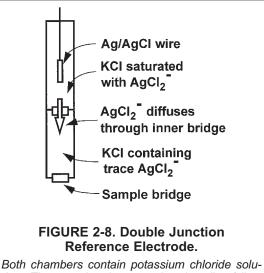
tion. The top chamber contains the silver/silver chloride reference element. The potassium chloride in this chamber is saturated with the soluble silver chloride complex. The silver chloride complex diffuses through the inner bridge into the second chamber. The concentration of the complex ion in the second chamber remains low, so the rate of pluggage in the sample bridge is slow.
