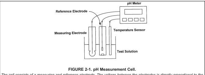
The construction of the electrodes and the electrical potentials associated with them are discussed in Sections 2.2 and 2.3.
