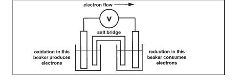
The voltage of the electrochemical cell (measured without drawing current from the cell) is the algebraic sum of the potentials of the two electrodes.
