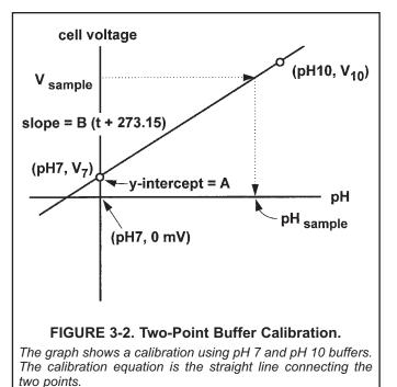
The microprocessor calculates the equation of the straight line connecting the points. The general form of the equation is:
