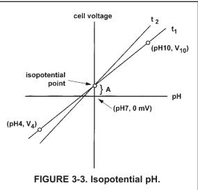
The graph shows two calibration lines. The original calibration was done with pH 4 and pH 10 buffers at temperature  $t_1$ . Suppose the temperature changes to  $t_2$ . The pH analyzer automatically changes the slope by the ratio  $(t_2 + 273.15)/(t_1 + 273.115)$ . The calibration equations rotate about the point (pH 7, A).
