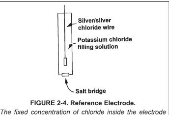
The fixed concentration of chloride inside the electrode keeps the potential constant. A porous plug salt bridge at the bottom of the electrode permits electrical contact between the reference electrode and the test solution.
