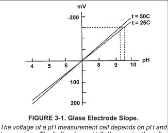
The voltage of a pH measurement cell depends on pH and temperature. The further from pH 7, the greater the influence of temperature on the relationship between pH and cell voltage.
