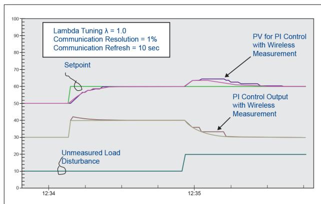
**Figure 1:** Control for wireless measurement is shown. All figures courtesy: Emerson Process Management from "Using Wireless Measurement in Control Applications," ISA 2013
