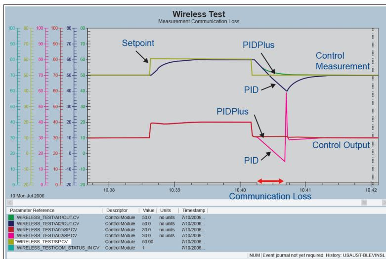
Figure 3: Response for measurement loss is shown. For the past four years, PIDPlus has been a standard feature of the DeltaV distributed control system. Emerson DeltaV users can select the PIDPlus capability as one of the control parameter options. Starting in fall 2014, Emerson is offering it free to WirelessHART users through the HART Communication Foundation.
