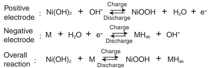
(M: hydrogen-absorbing alloy; H<sub>ab</sub>: absorbed hydrogen)
