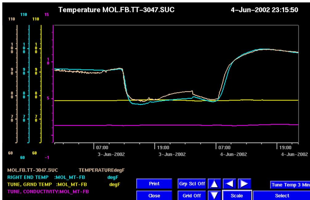
Figure 6. Trend of Measured Temperature and Calculated Temperature at Fourchon Station
