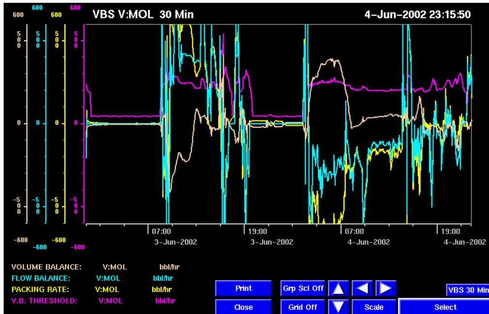
Figure 10. Leak Alarm Generated by the Model. The configuration is set with a very low heat capacity (20 times smaller than normal).
