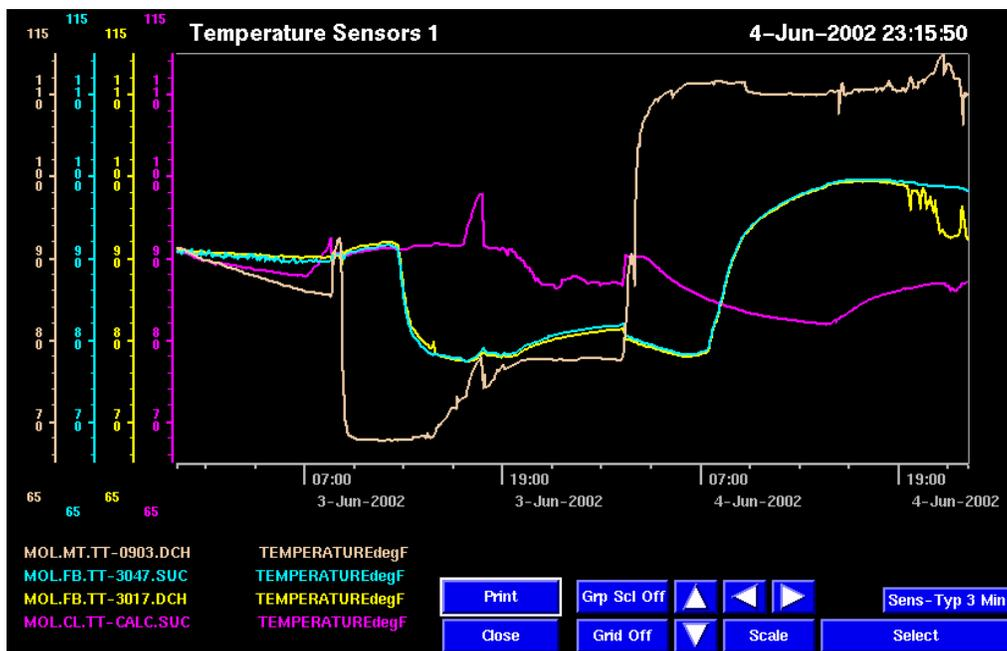
Figure 5. Trends of Temperature Measurements at 4 Points in the Line
