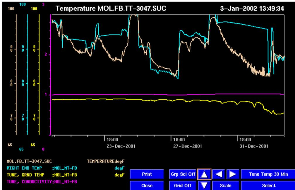
Figure 11. Trend with Measured and Calculated Temperatures during Numerous Shutdowns
