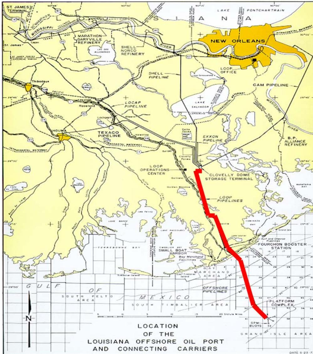
Figure 1. Path of LOOP Pipeline
