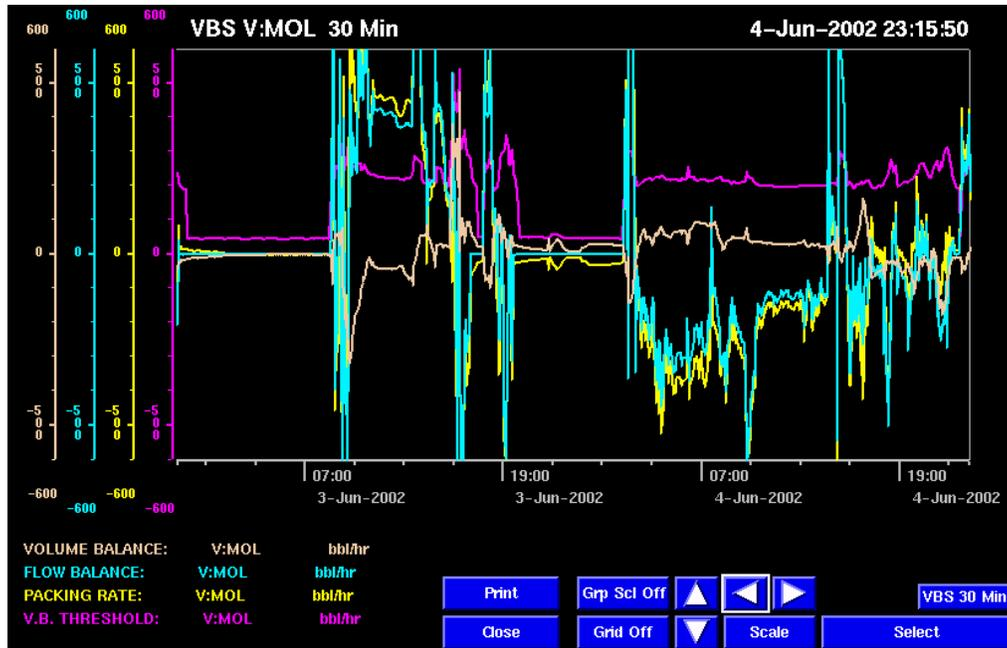
Figure 7. Leak Detection Trend, Tracking is Good with No False Alarms
