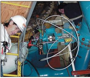
Fig. 2. Control valve instrumented for test
