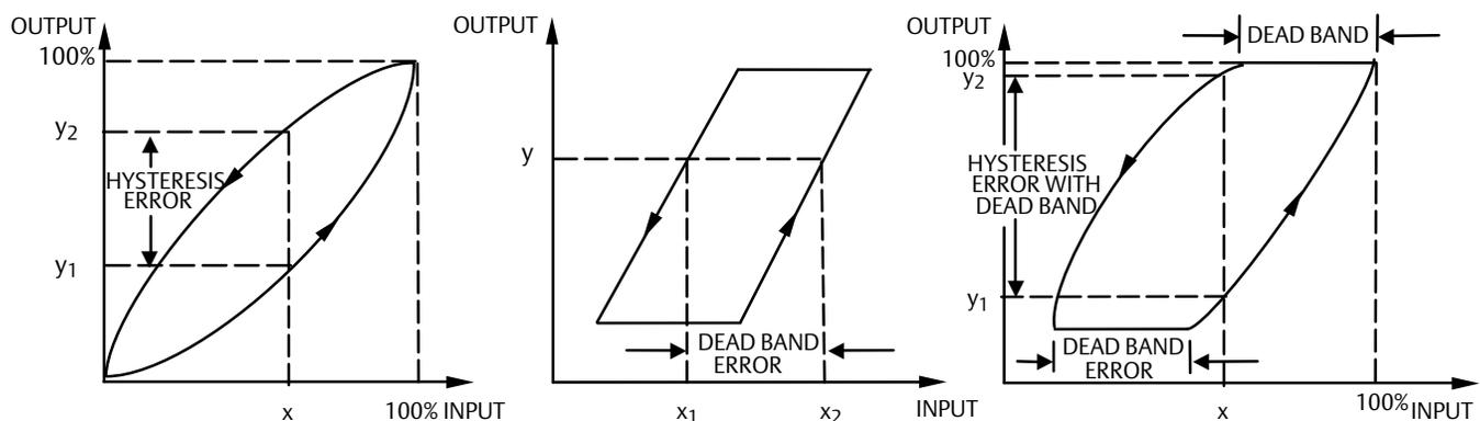
For control valves, dead band is the dominant nonlinearity whereas hysteresis is a secondary effect. Hysteresis can be estimated by subtracting dead band from the dead band plus hysteresis data. However, since hysteresis is generally negligible and difficult to discern from experimental error, dead band and hysteresis are not separated and test results are reported as the sum of these nonlinearities.
