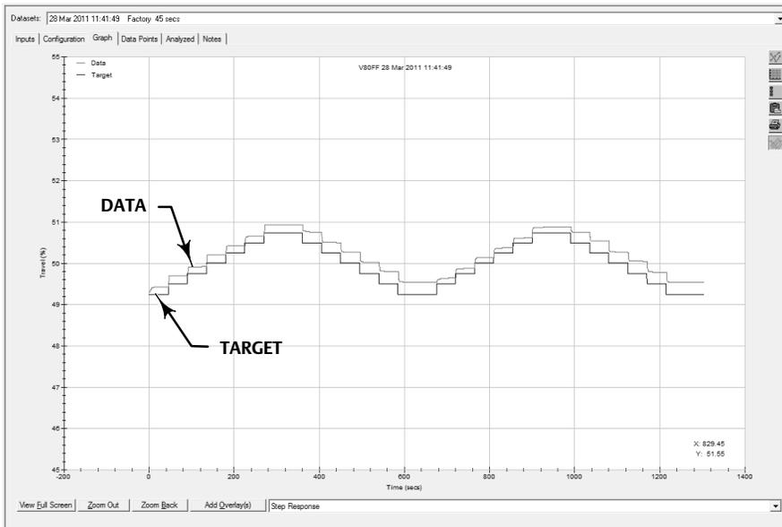
Note: The first cycle is a break-in cycle. The second is a test cycle.
