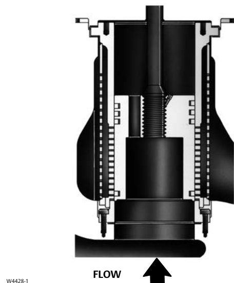
Figure 11. Fisher EHD Trim with Whisper Trim III Level D Cage (NPS 8 through 14 Globe Valves)
