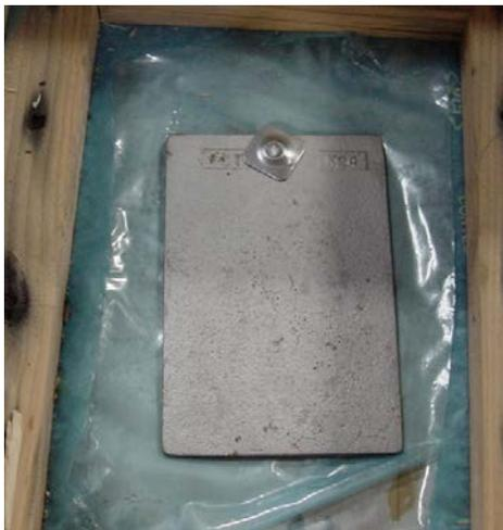
Figure 3 packaging method utilized Cortec VpCI-126 polyethylene under and over the test panel. The panel was sandwiched between the two VpCI impregnated polyethylene layers. Frame lumber was nailed to hold the sheeting in place. The container was built with uprights, but no barrier material was used over the skid framework sides, ends, or top. The panel is virtually rust-free.
