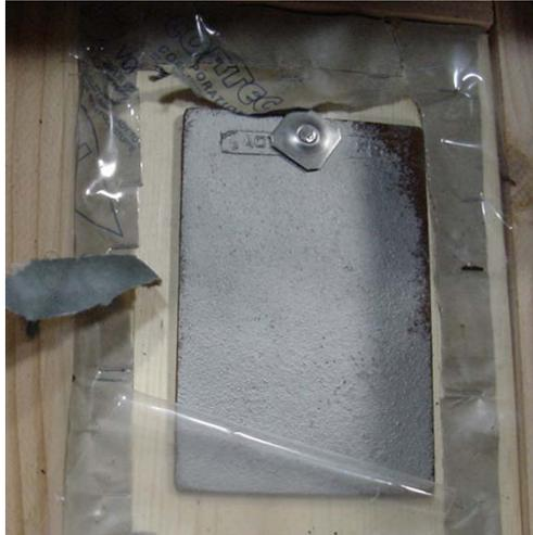
Figure 1 packaging method utilized tarpaper under the panel and the container uprights covered with tarpaper with seams glued. The panel was covered with VpCI paper and plain plastic sheeting (not VpCI plastic). Heavy rust is visible on the upper right side of the panel.
