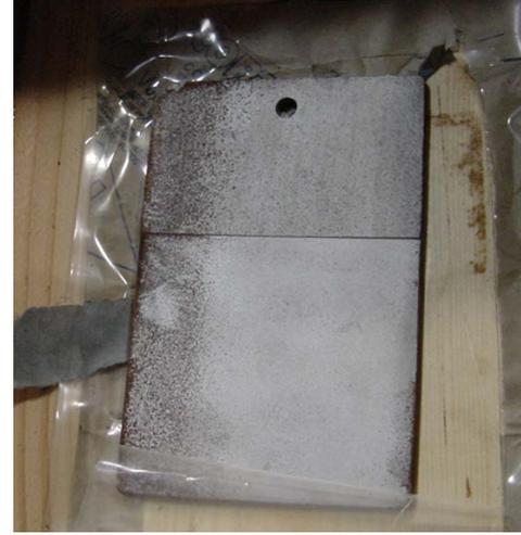
In figure 2, square headed nails were removed from the panels and the panels were turned over. With the old tarpaper method, the same side that was heavily rusted in figure 1 now exhibits heavy rusting on the under side (left side) of the panel. Rusting has begun on the opposite side as well.
