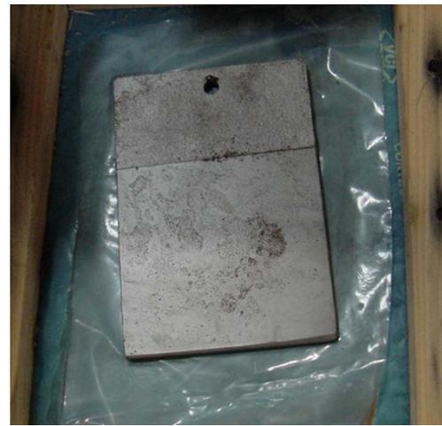
In figure 4, some minor rust is visible on the underside of the panel protected with Cortec VpCI-126 poly, but the largest area of this rust appears to be from a thumbprint or fingerprint.
