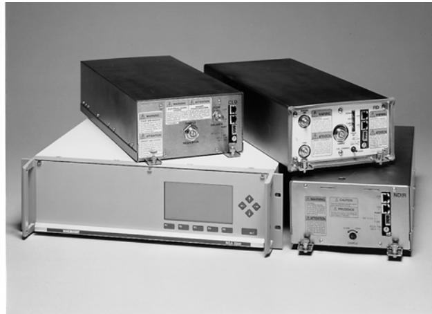
Emerson's Rosemount Analytical NGA CLD NO/NO<sub>x</sub> analyzer module was the industry's first modular chemiluminescence analyzer. It is a self-contained unit complete with detector and electronics. The modular design allows for easy system integration. The CLD analyzer module may be a "stand alone" analysis instrument with the addition of our input/output (I/O) module and platform or it can be integrated into a sophisticated multi-component analysis network.
