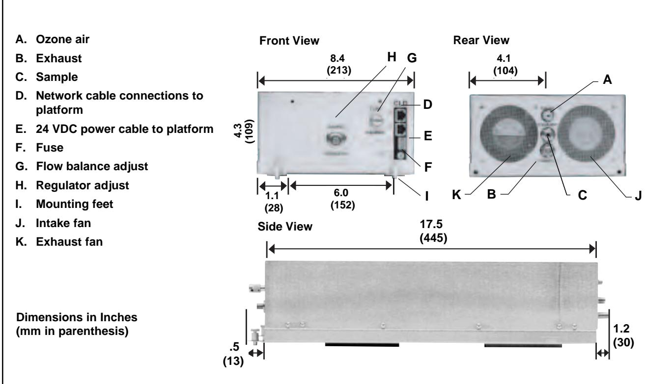
Platform with internal analyzer module. Several analyzer modules may be integrated with a single platform, either mounted inside or located externally. (Platform shown here with top removed.)
