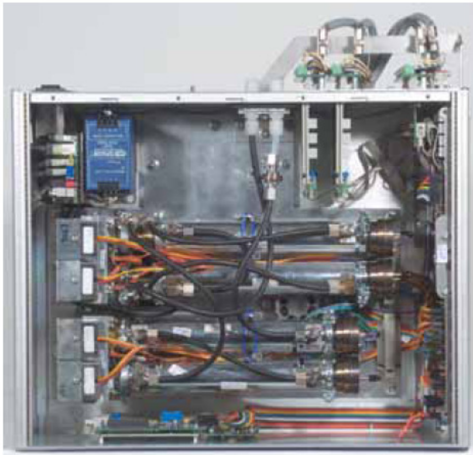
Interior view, showing 4 NDIR benches, thermostatic control (cover removed), analog and relay outputs, digital inputs, and serial interface.
