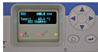
The alphanumeric display of the X-STREAM X2 provides measurement and status information with plain text on either an LCD or VFD, supported by LEDs.
