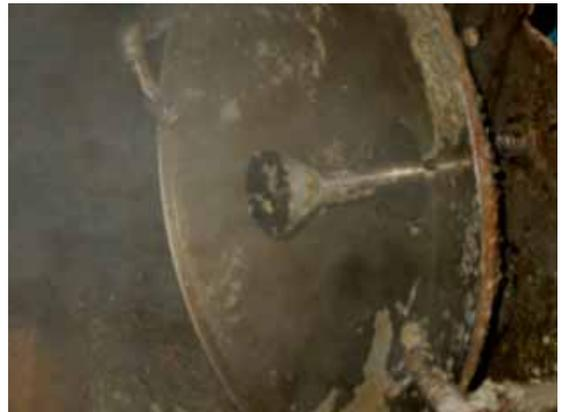
*Parabolic Antenna covered in pulp stock. Flushing lines for cleaning are installed near the edge of the dish.*
