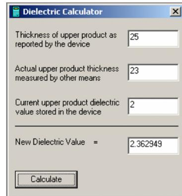
*The dielectric calculator in the Radar Configuration Tools*
