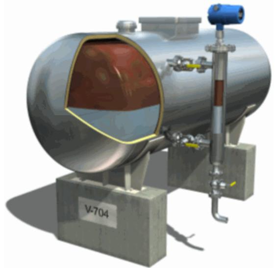
measurement mode, the probe length, the range values and the dielectric of the oil. To determine the fluid dielectric, the water was temporarily removed and the chamber was flooded with oil. While in this condition, the peak created by the end of the probe (a known distance) and the dielectric calculator in Radar Configuration tools were used to determine the dielectric.
