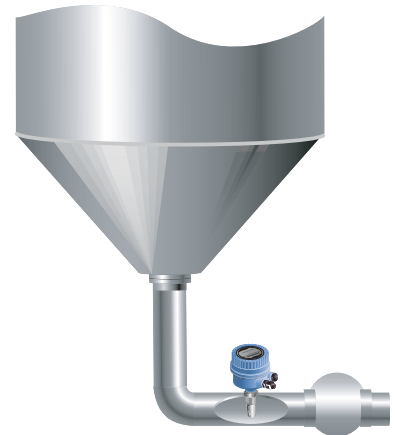
Rosemount 2120 mounting for successful low-level drain.
