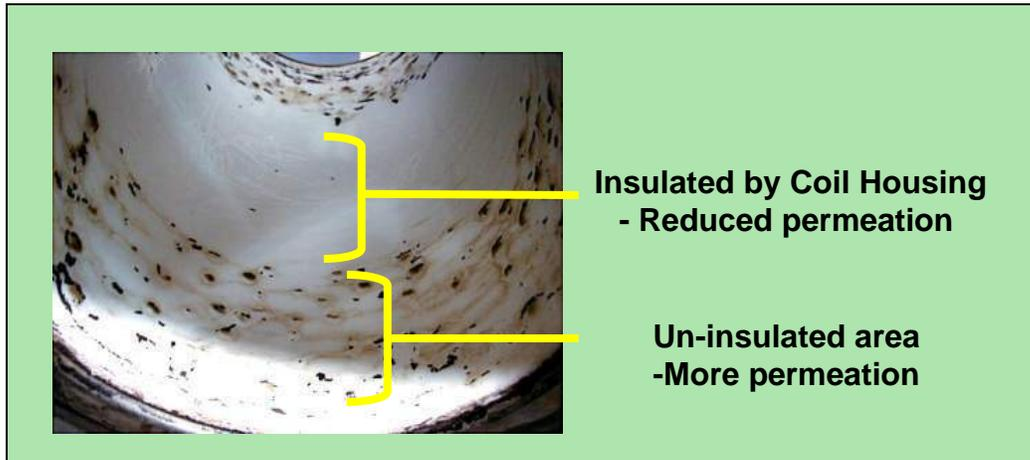
Teflon Blistering in Insulated and Un-Insulated Meter Sections
