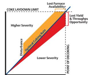
Emerson's SmartProcess pyrolysis furnace application provides control functions designed to maximize the yield of high-value products from each of your cracking furnaces. Improved control of furnace severity, charge rate and dilution steam ratios, combined with pass outlet temperature balancing, ensures furnaces can be operated at maximum severity and still achieve your desired run length between decoking cycles.
