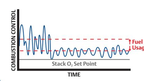
While pyrolysis furnaces are generally designed to be highly efficient, you can further boost efficiency by using stack O<sub>2</sub> and CO analyzers to minimize excess air, variable speed drives for induced draft fans, and abnormal situation prevention (ASP) techniques to detect flame instability.
