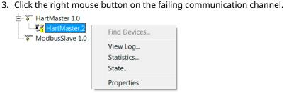
4. Choose the **State** option to find out which device that is not properly communicating on the HARTMaster channel.
