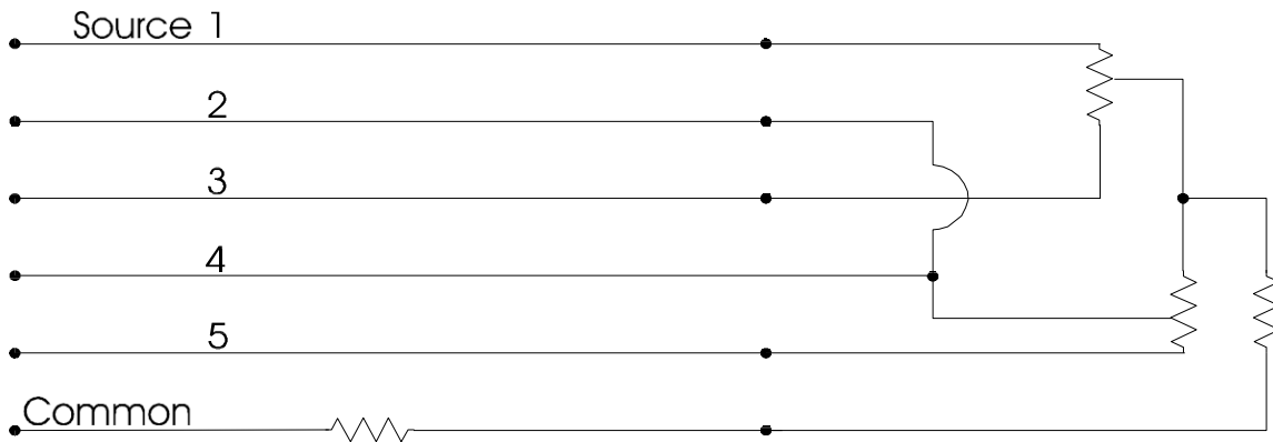
Figure 5-2. Field-wired Circuit with a Common Return
