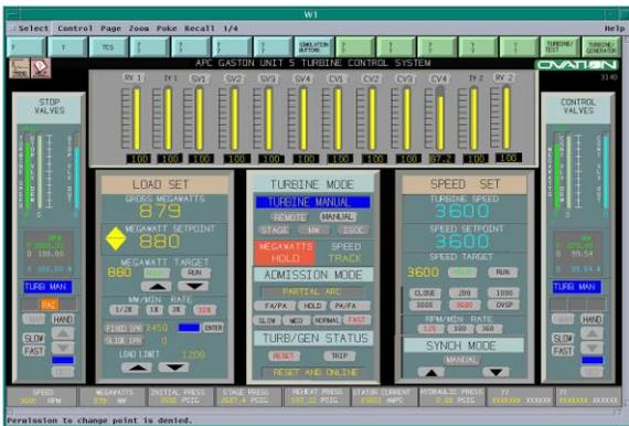
The Emerson steam turbine package performs all the original GE control and protection functions. Normally included with this solution is:
