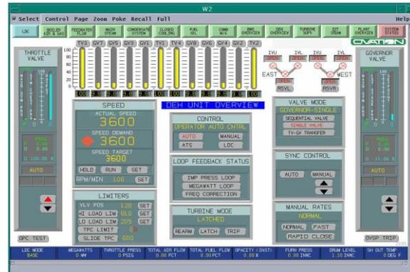
The Emerson steam turbine package performs all the original Westinghouse AEH or DEH overspeed protection and operator automatic control functions. Protection and testing functions normally include:
