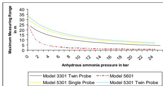
Measuring range in bar versus meters
