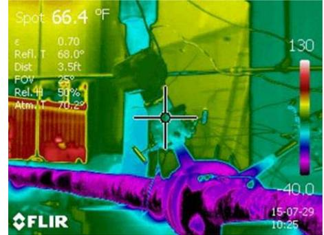
FLIR image of flowmeter during cryogenic testing
