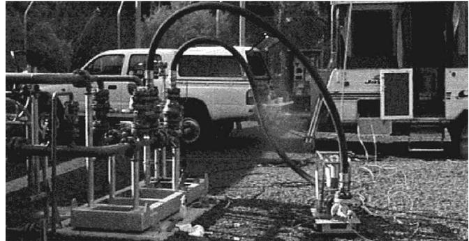
Figure 3. Portable Proving Meter
