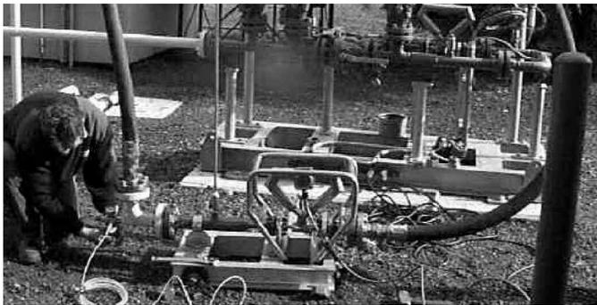
Figure 2. Portable Proving Meter and Proving Caravan
