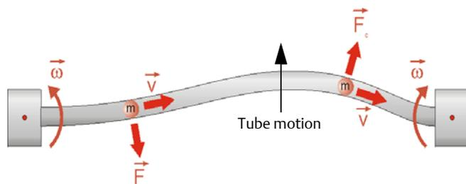
Figure 2. Coriolis "twist"
