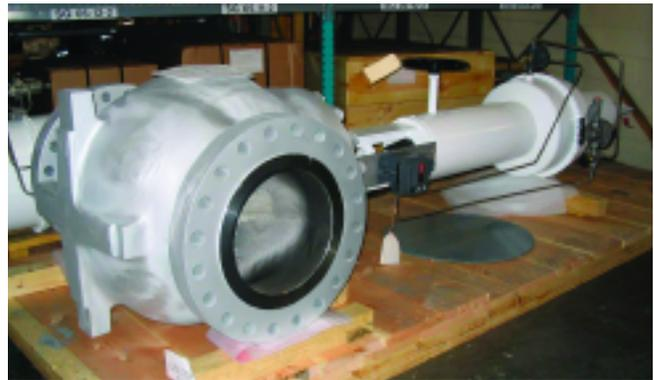
*This Fisher® valve assembly, bound for Kazakhstan, was 13-feet long with a DVC6000-PD, Type 3025 actuator, and a hand-wheel enabling manual on/off.*
