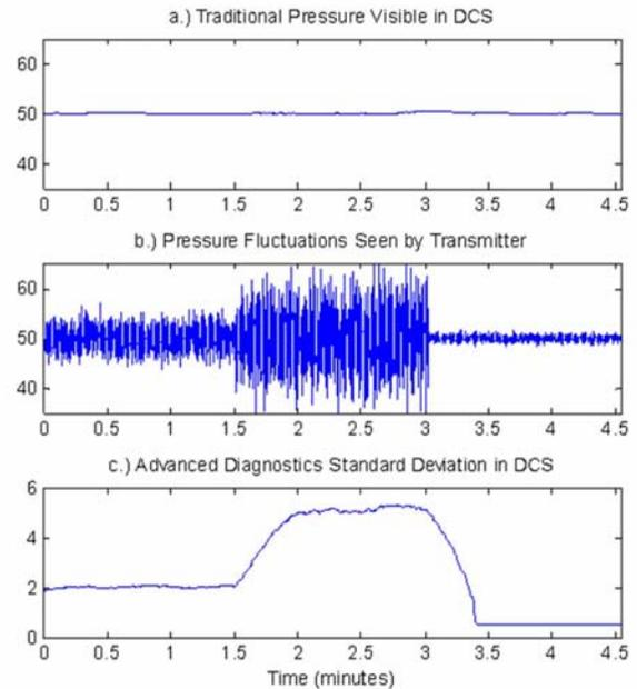
FIGURE 2. Trend of Advanced Pressure Diagnostics Data
